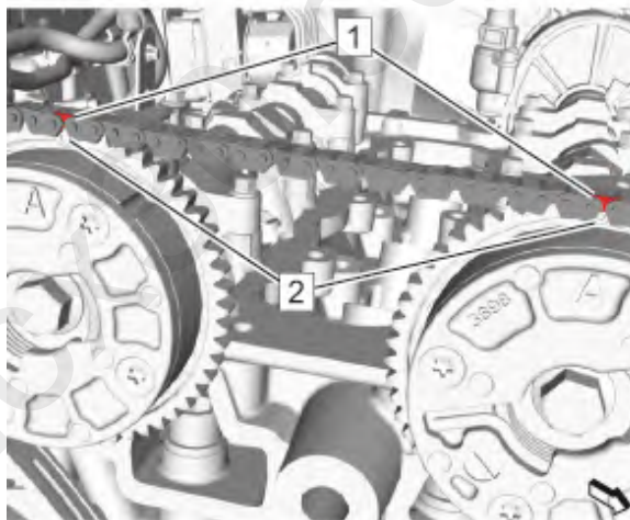
Fig. 63: Camshaft Position Actuator Marks And Timing Chain Marks Courtesy of GENERAL MOTORS COMPANY
